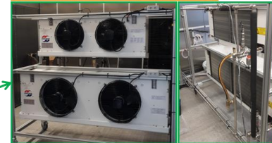
Evaporators Chamber B
